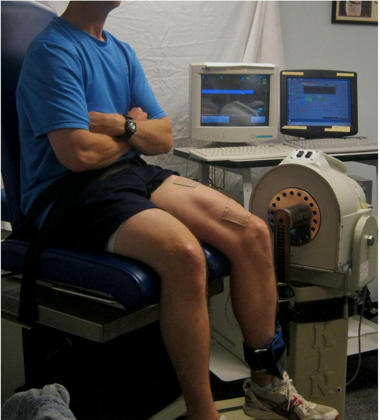
**Figure 1.** Maximal volitional isometric contraction of the quadriceps with burst superimposition testing.
